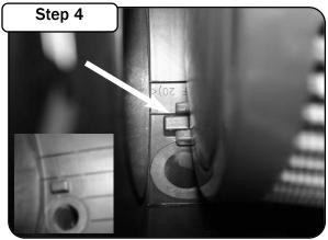
Notice the square tab at the bottom of the airbox. The pronged post should capture this as shown.
