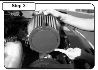
Notice the difference between the posts on the fil-ter. The post with the two prongs is pointed down and should be inserted into the air box first. Tilt and slide down.
