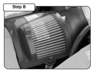
Screw the air filter cover down. Verify the air box cover closes correctly. Your installation is now complete.
