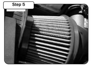
It will be necessary to tilt the filter to align the pronged post with the air box tab and then angle the filter into the OE air box.
